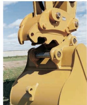
Pin Grabber Plus Hydraulic Pin Grabber
